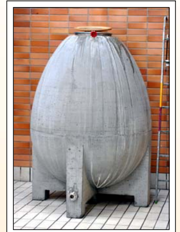
Abb. 1 Beton-Ei (900 l, 1800 kg)
